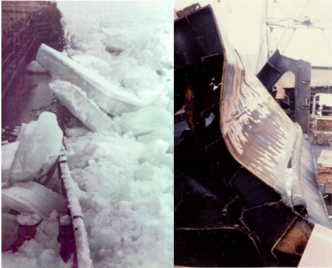
Figure 1.1: A ship stuck in compressive ice and the damages that resulted from the ice load. (Riska, 2011)
