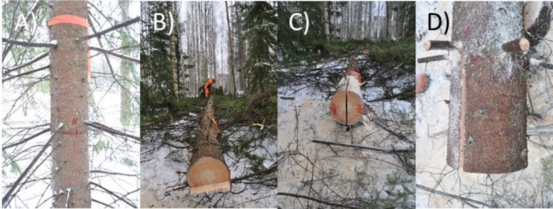
Figure 10. From left to right: A) marking the compass direction before felling, B) trimming the tree and marking 20 cm samples for every meter up to 10 m height, C) keeping track of north and south sides, and D) finally slicing the 20 cm length log to produce two samples per meter of height.
