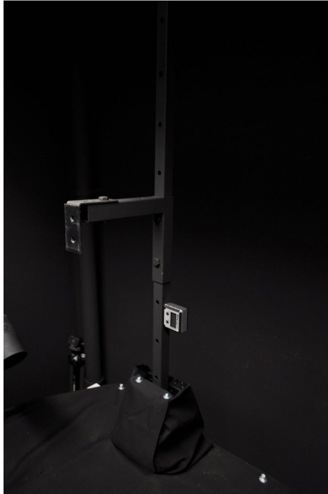
Figure 2. The goniometer arm combined with an L-shaped bar with attachment possibility for sensors at the end of it. Machined holes at 10 cm intervals visible in the picture allowed the measurement height to be adjusted if needed. Small square apparatus attached to the side of the arm was a digital angle gauge.
