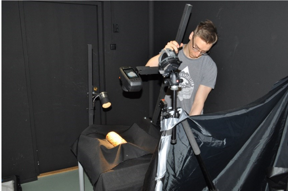
Figure 7. The multi-angular measurement setup with a sample under investigation. The setup consists of the lampstand integrated with the aluminum beam restrictor with a halogen lamp inside, the multi-angular system with black coating on top, arm lever that can be rotated 180 degrees that also has the sensor attached to it (Specim IQ), laboratory room painted black, a laser pointer and extra curtaining. Actual measurement was done with the external lights turned off.
