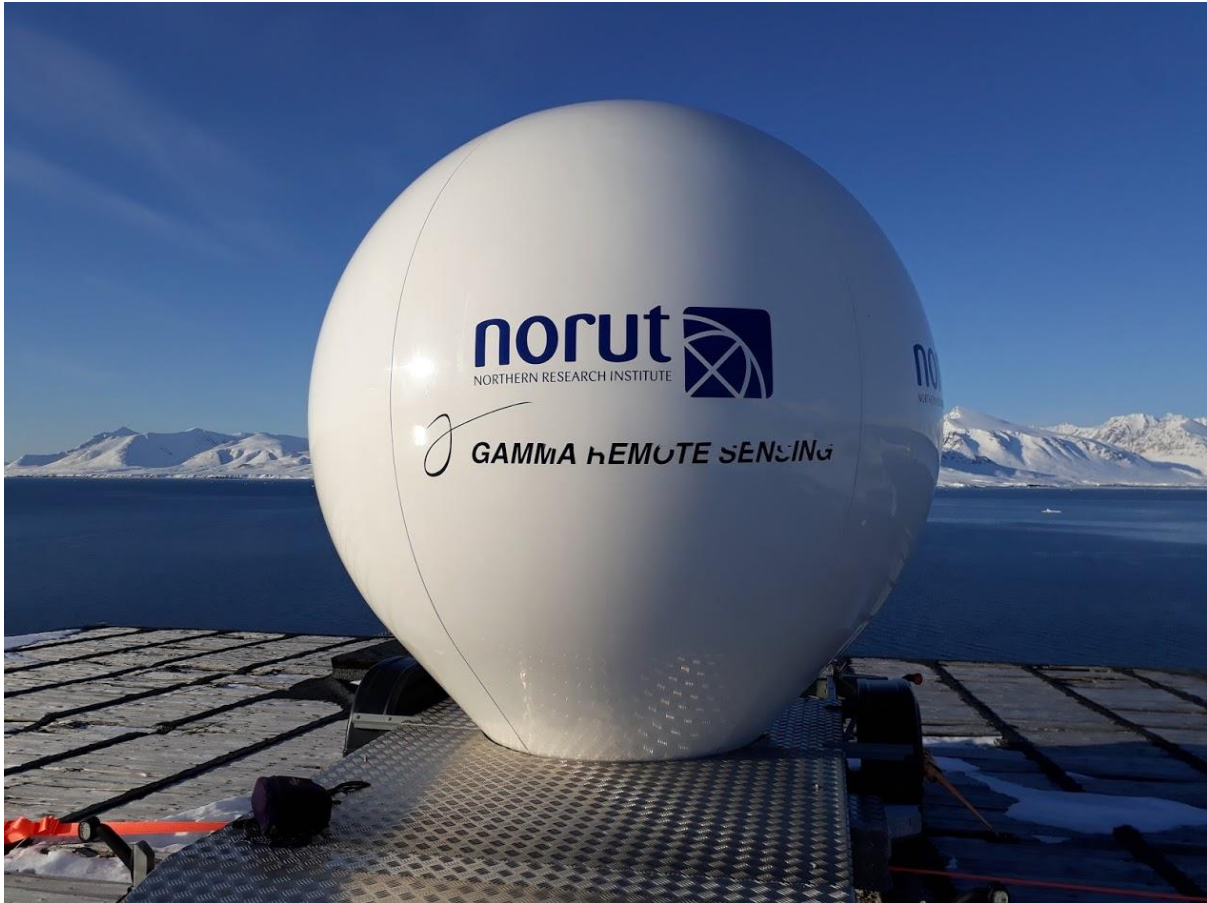
Figure 7: The radome protecting the GPRI facing Kongsfjorden in Ny-Ålesund (photo taken by Line Rouyet 25.04.2018).
