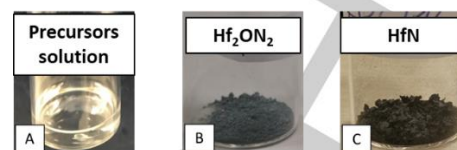
Figure 12. Photographs showing the precursor solution (A), the final product obtained after heat treatment under N 2 flow at 900 °C (B) and 1200°C (C), respectively. Phase attribution was made by PXRD study (see text for details).
