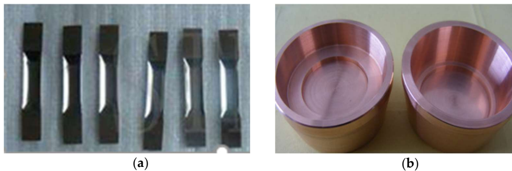
Figure 4. (a) Molybdenum boats for thermal evaporation; (b) crucible for electron-beam (EB) evaporation.
