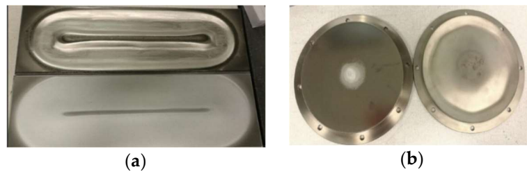
Figure 5. (a) Racetrack shape in rectangular sputtering target; (b) racetrack in circle shaped target.
