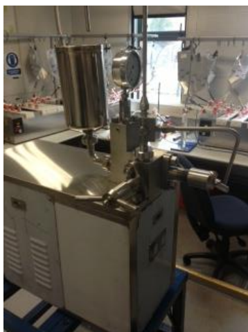
Figure 1: GYB40-10S 2 stage Homogenizer Figure 2: HPH parts during cell disruption [22]
