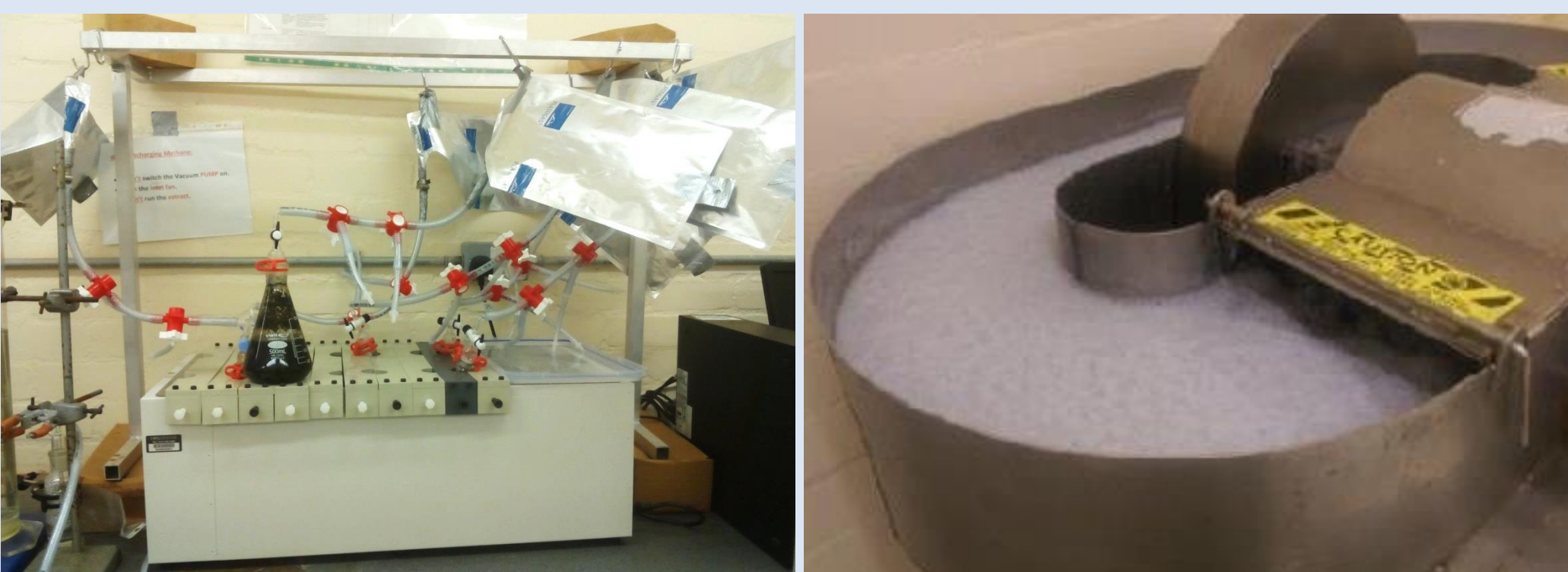
Fig. 2. Bioreactors setup (left) and Hollander beater used in this study (right)
