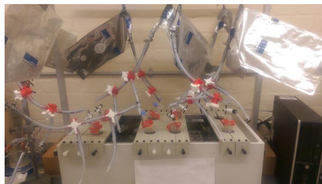
Figure 2. Reactors with collection systems.
