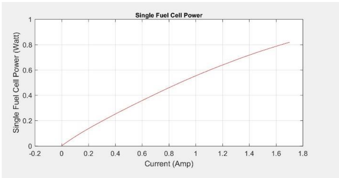
Figure 17a: Plot of Power and current from one cell stack.
