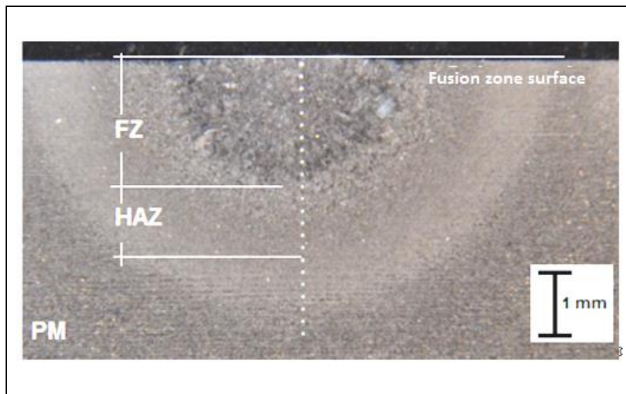
Figure 3. Pattern of indents taken on cross- sectional area of melted track. First indentation taken at 0.1 mm from the fusion zone (FZ) edge and 0.2 mm apart towards the parent material
