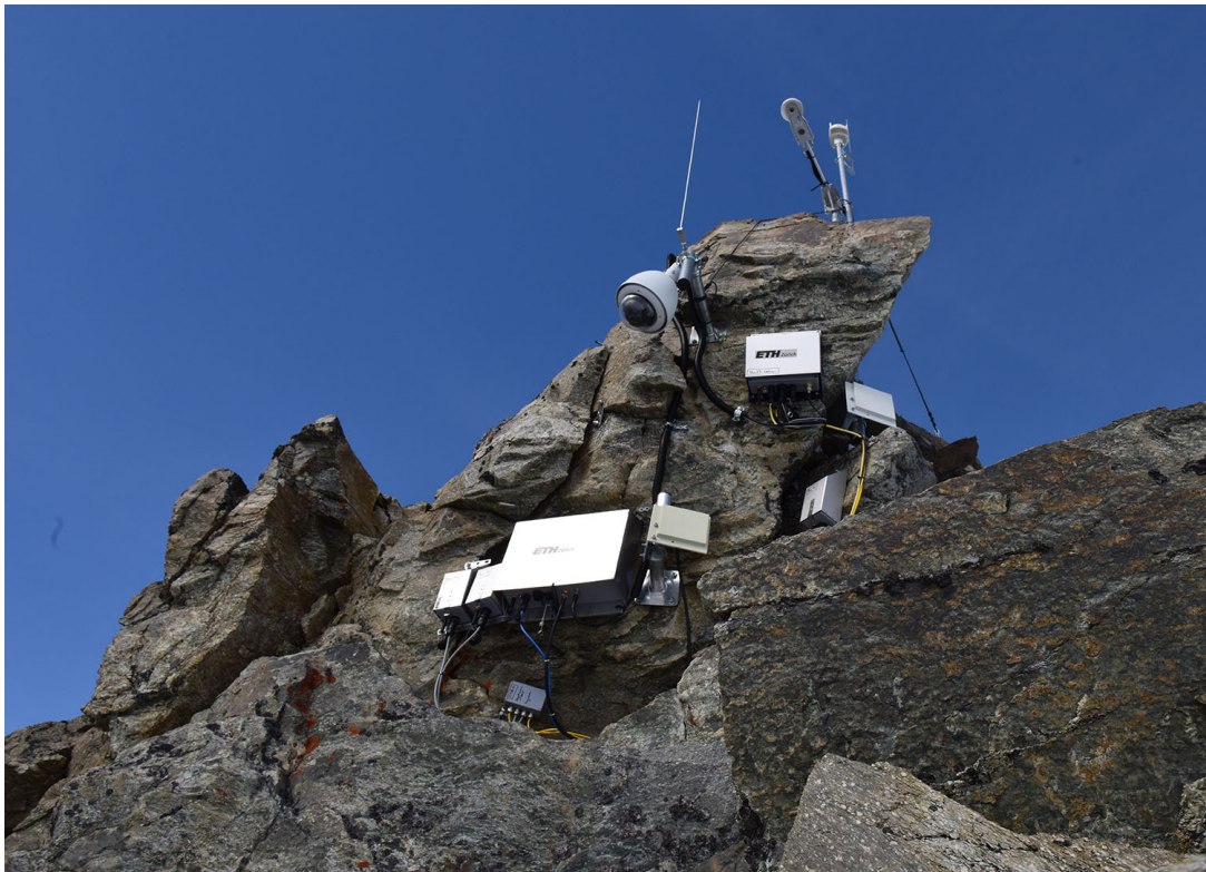
Figure C4. A Vaisala WXT520 weather station and Kipp & Zonen CNR4 radiometer are installed on top of the ridge crest. Other equipment shown here are a webcam, Leica GRX1200+ high-precision GNSS receiver and the required wireless transmission and power control equipment.
