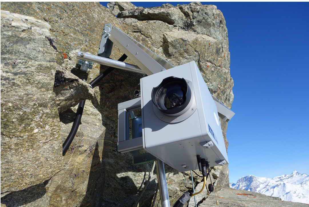
Figure C8. High-resolution time-lapse camera located at position MH19.
