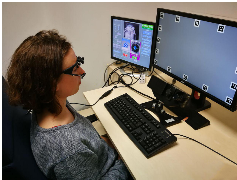
Figure 1 Experimental Setup. The remote eye-tracker EyeLink 1000 is located beneath the computer screen that displays the stimuli. The participant wears the mobile Pupil Labs glasses. The auxiliary calibration monitor on the left was turned off during the experiment. (Photography Katharina Groß; subject's consent to publish this image was granted). Full-size DOI: 10.7717/peerj.7086/fig-1
