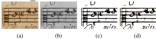
Figure 3. Examples of the pre-processing transformations applied to the input staff sections: (a) Original RGB image, (b) Grayscale, (c) Binarization, (d) Channel-wise binarization. This figure must be seen in color.
