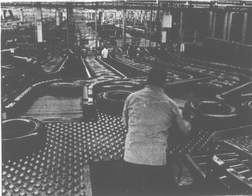
ROLLING OUT THE TIRES—Some of the 33,000 tires produced each day in Goodyear's Union City plant are sorted in the Final Finish Department by Bill Miller. All production
