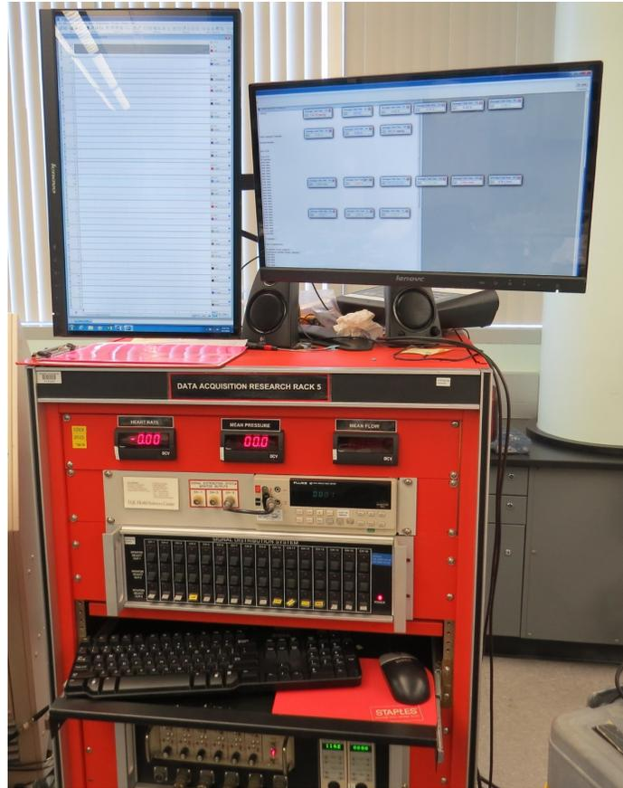
Figure 13. Data acquisition system (DAQ) with LabChart software used throughout the experiment to record hemodynamic waveforms.
