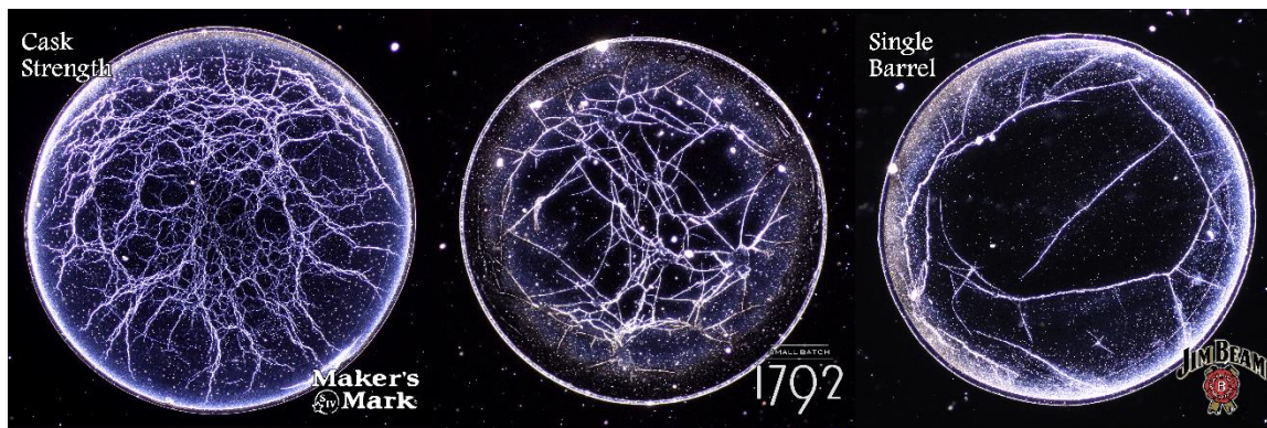
Figure 8 - Whiskey webs a) Maker's Mark Cask Strength™ b) 1792 Small batch™ c) Jim Beam Single Barrel™. The web patterns shown appear different in nature, this observation has been validated by numerous qualitative experiments. Figure reproduced from (Brown, et al. 2019).
