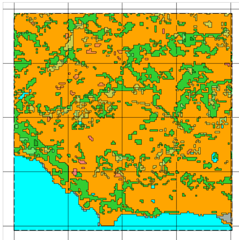
Figure 14. Roughness map of the area around the meteorological mast WM05, Napier. The map covers an area of 40x40 km 2 and the land cover classification is from ESACCI 2015 data.
