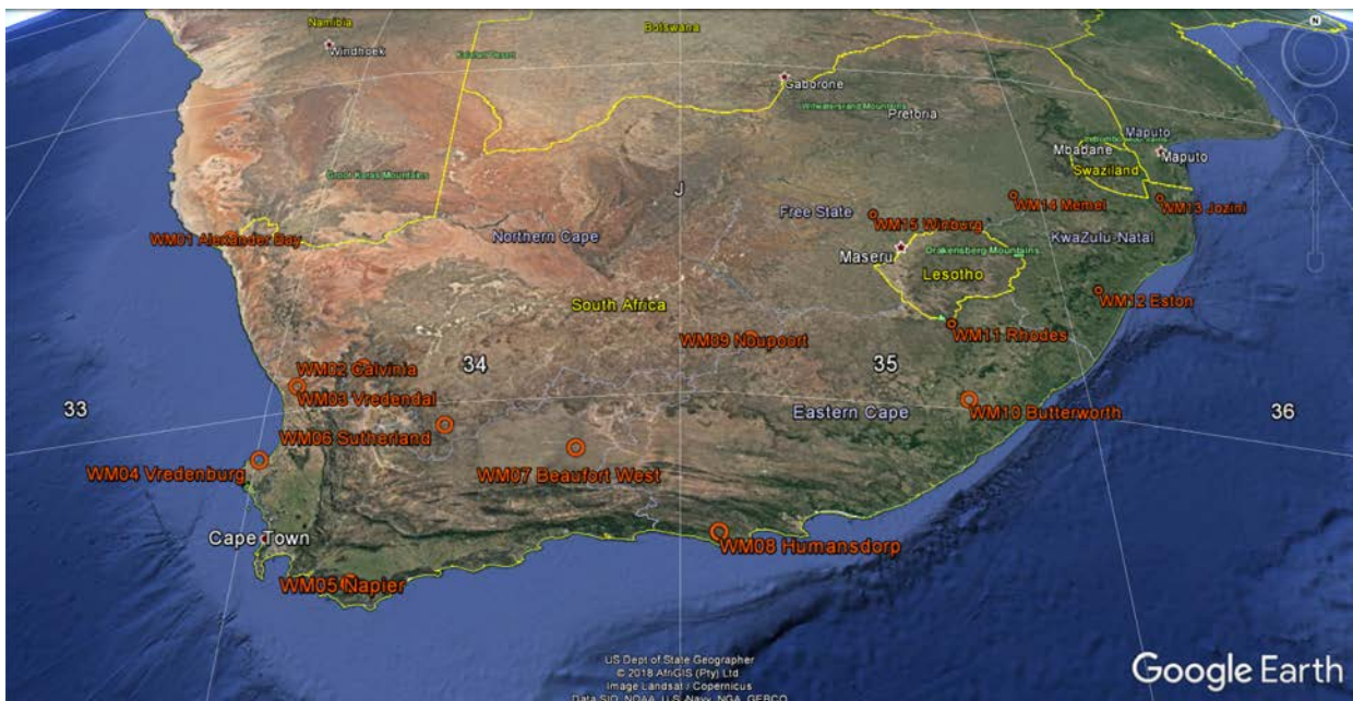
Figure 16. Google Earth image of southern Africa showing the three UTM zones covering the WASA Phase 1 domain: 33, 34 and 35. Each zonal coordinate system is Cartesian and the coordinates can be given in [m] or [km].
