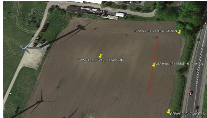
Figure 1: Position of the three short-range WindScanners and the reference meteorological mast located east to the V52 turbine (left). The red line symbolizes the lidar scan plane.
