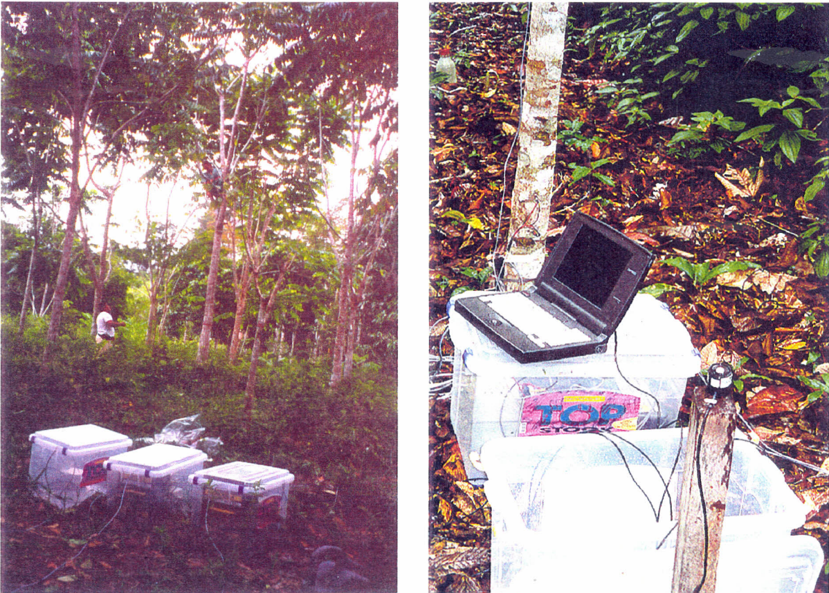
Fig. 1a/b: Installation of xylem flux sensors at the experimental plots in Manaus.
