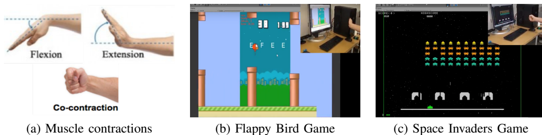
Fig. 1: (a) Three main muscular contractions (flexion, extension, co-contraction) used to control a robotic prosthetic arm and Game screens of (b) Flappy Bird and (c) Space Invaders in our training tool.
