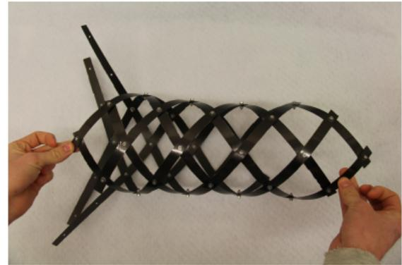
Self locking end constraints and friction causing problems.
