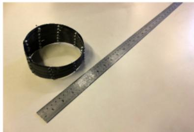
A helical lattice balancing effects of pre-stress, material properties and geometry, was constructed [Pirrera *et. al.* (2013)]
