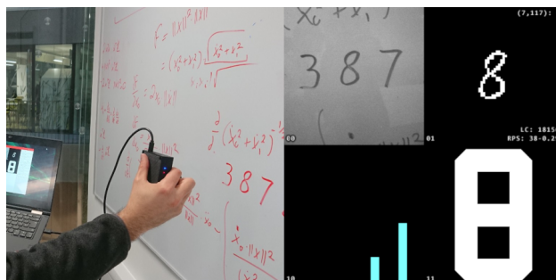
Figure 1: The SCAMP5, a sensor-processor that does true end-to-end capture and processing with a CNN on its massively parallel pixel-processor array. Here it demonstrates digit prediction from hand-drawn input (left) using inference of a MNIST trained CNN to produce the correct output (bottom-right corner).
