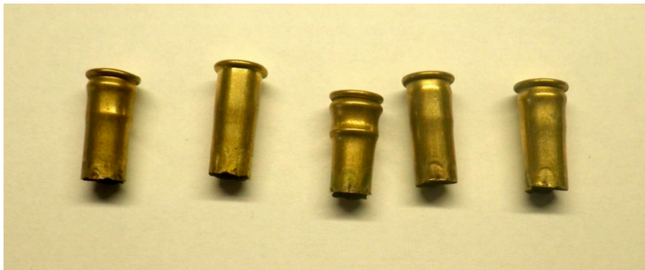
Figure 18. Range of deformities seen in cartridge cases fired using the same device.
