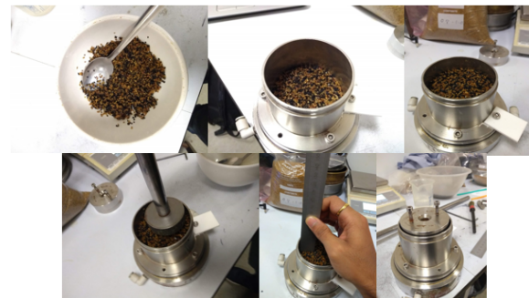
Fig. 3. Figure showing the preparation of sand-rubber mixtures using moist tamping method
