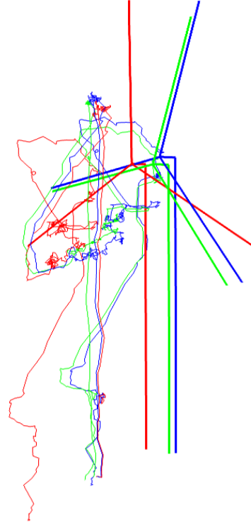
Fig. 5. Visual example of the combined pose and model optimisation process. The green turbine corresponds to the ground truth \mathcal{P} , the red to the initial configuration of \mathcal{P} and the blue to the optimised configuration of \mathcal{P} . Similarly, the green path corresponds to the ground truth positions of the drone, the red to the initial positions and the blue to the optimised positions.
