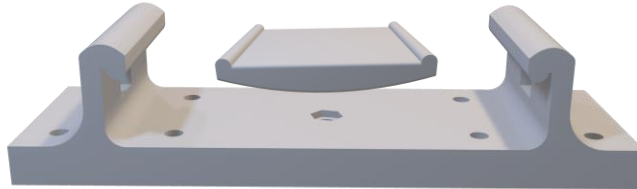
Figure 53 New four-point bending specimen design with much more less material.
