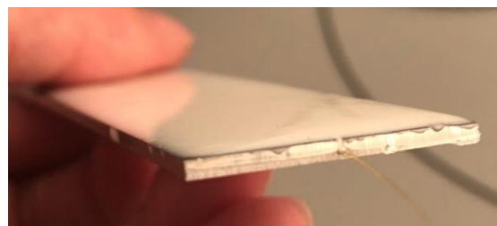
Figure 29 low-carbon plate with FBG embedded in and anti-corrosion adhesive layer at one side.
