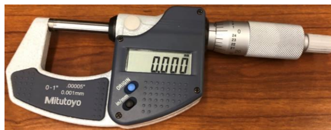
Figure 51 Spiral micrometer used for measuring the thickness of the corroded areas.
