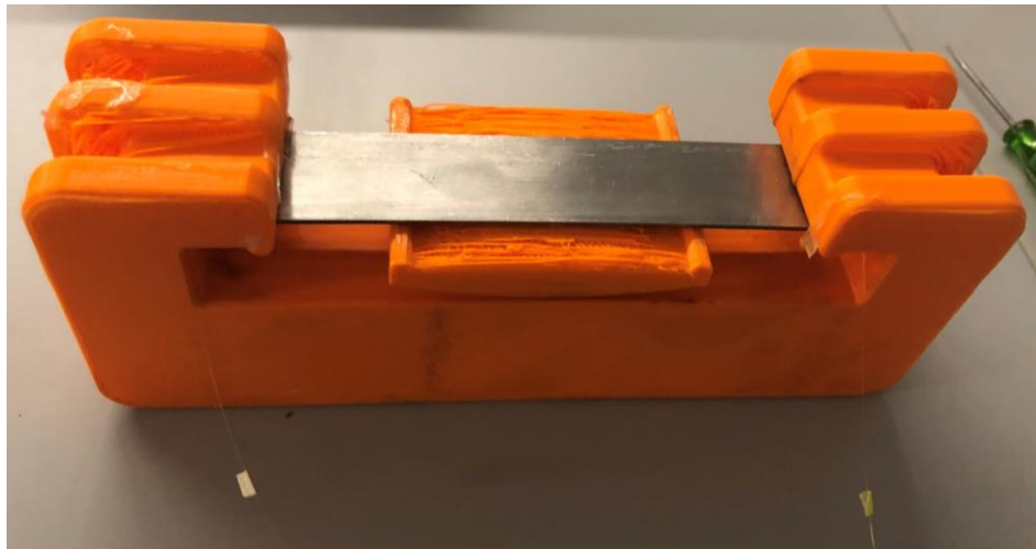
Figure 32 Four-point bending specimen with low-carbon steel installed on, with screw upward 2.5mm.
