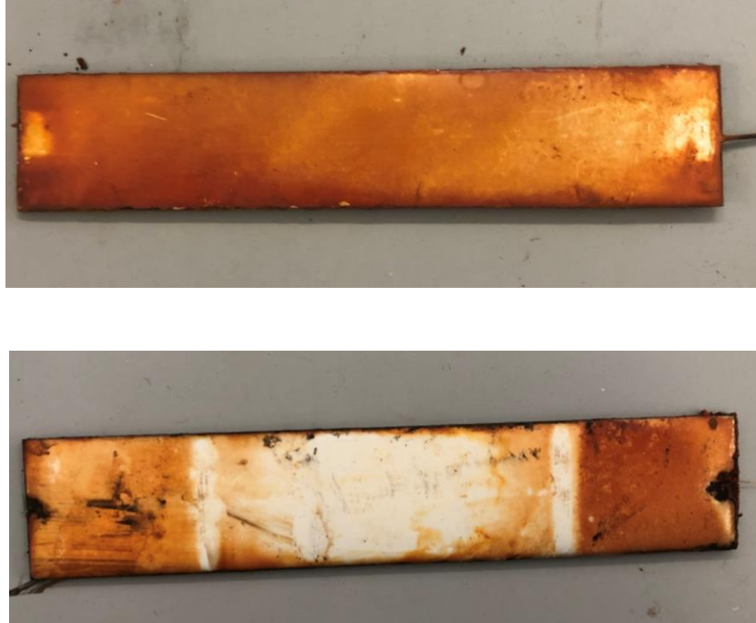
Figure 41 The coating layer made by so called high corrosion resistant changed after long time corrosion.
