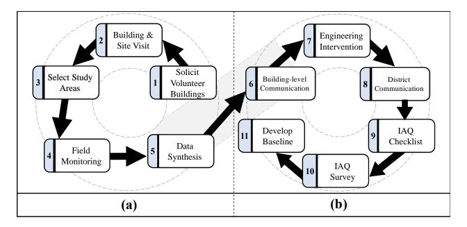
Figure 2. Eleven steps of indoor air quality framework - Indoor air quality framework broken down into two parts, the a) detailed sampling procedures and b) feedback and remediation.
