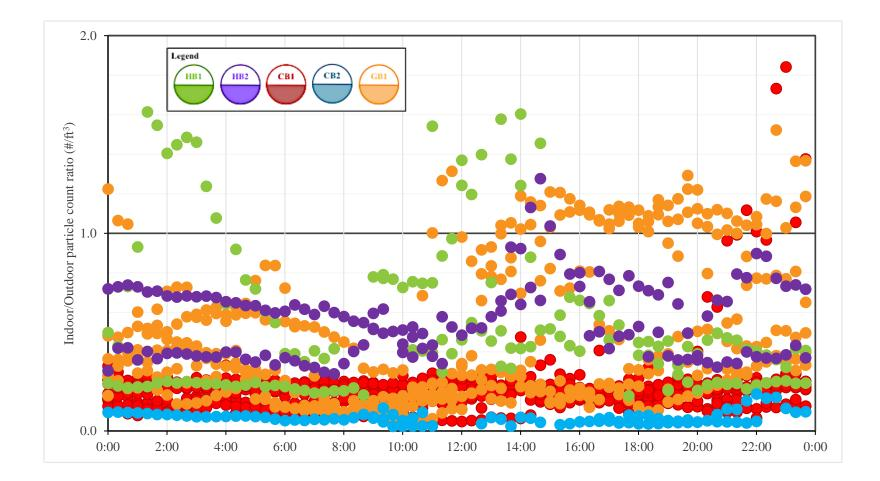
Figure 7. Indoor to outdoor ratios of PM across five pilot buildings - I-O PM counts for the smallest size bin for PM (0.3 – 0.5 μm) of five of the eight pilot buildings over a 24-hour period. The buildings are identified with a unique code where the first two letters represent the archetype (i.e., historic building (HB), conventional building (CB), green building (GB)) and the number is a differentiation for each building in the pilot.
