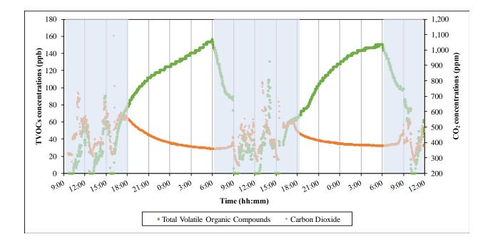
Figure 8. TVOCs and CO<sub>2</sub> concentrations in Building GB1 - Results reflect data during hours of operation and overnight.
