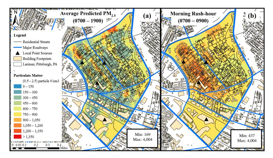
Figure 11. Average Predicted PM<sub>2.5</sub> Dispersion Map - 853, 318, and 424 particle counts (particle #/cm<sup>3</sup>) were recorded during the morning, afternoon, and evening sampling period, respectively.
