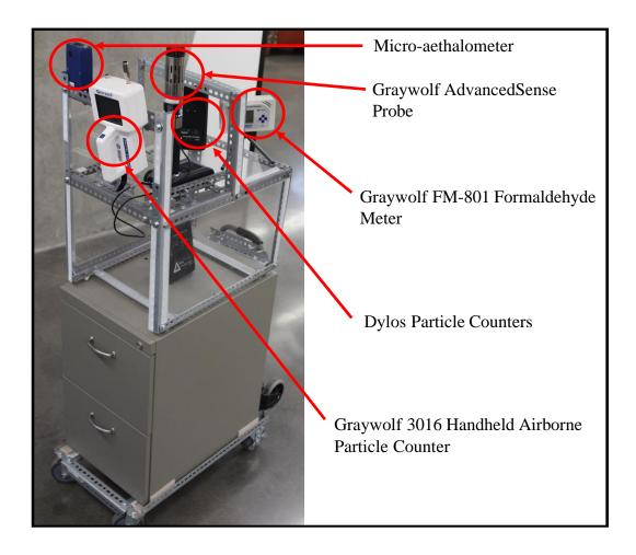
Figure 19. Mobile indoor air quality cart. A mobile cart was configured (a height of 1.5 m), which housed the
