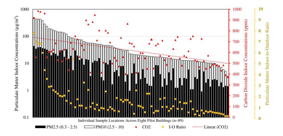
Figure 6. PM<sub>(0.3-10)</sub>, CO<sub>2</sub>, and PM indoor-to-outdoor ratio and spot measurements - Indoor-to-outdoor ratio and spot measurements represent a duration of 30 minutes across three-days, at individual test locations in the eight pilot building.
