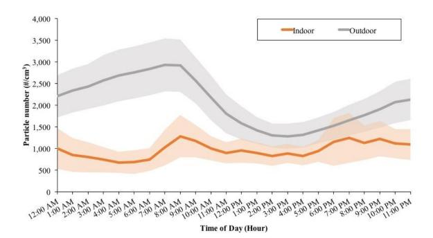
Figure 16. Comparison of indoor and outdoor PM<sub>2.5</sub> concentrations - Combined PM concentratins from both EJCAM and ROCIS by time of day averaged across 51 sample homes; line plot bands represent 95% confidence interval.
