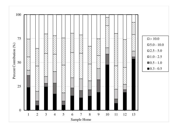
Figure 15. PM indoor concentration by bin distribution - Contribution of indoor particle mass concentrations displayed as percentage of total mass concentration sampled.
