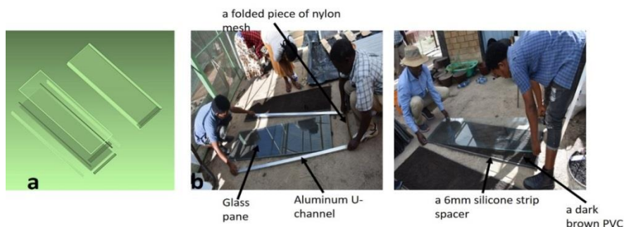
Figure 1. Showing top view of rhizobox diagram (a) and components of rhizobox (b)
