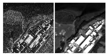
Figure 1. Comparison between acquired SAR (left) and optical (right) images.
