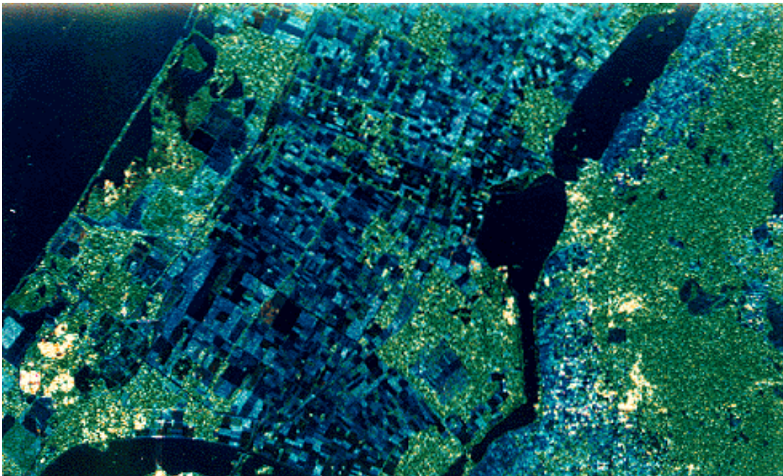
Figure 4: The Freeman-Durden decomposition applied to L-band SIR-C polarimetric SAR data over the Flevoland supersite, in the Netherlands. Blue = surface scattering; Red = double-bounce; and Green = Volume scattering. Areas that show up yellow have strong double-bounce scattering, mixed with volume scatter.
