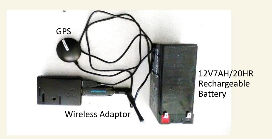
Figure 1. gBT system components
