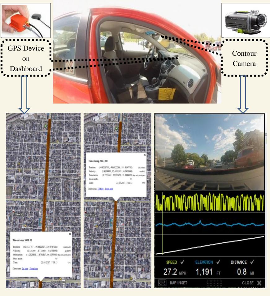
Figure 3: Test vehicle setup showing (a) GPS trajectory with time stamps, and (b) speed profiles
