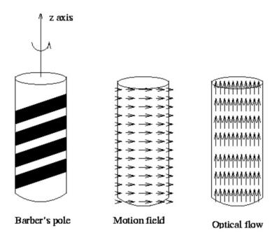
Figure 2.8: Motion vectors of moving barber's pole
