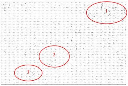
Motion vectors using Horn and Schunk method
