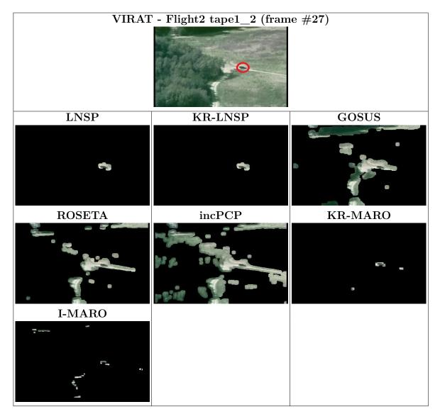
Figure 5.13: Sample results of the compared PCP detection methods on VIRAT
