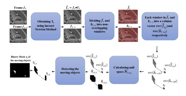
Figure 5.2: Detecting moving objects based on multiple local null spaces
