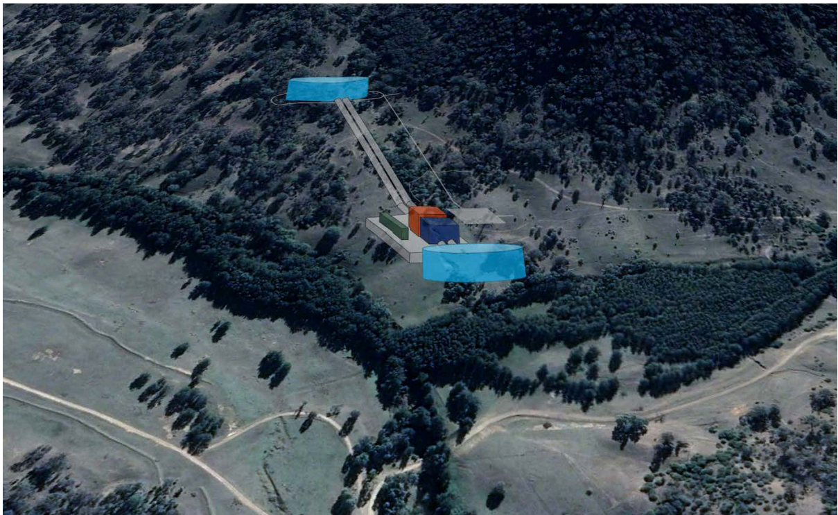
Figure 25: Google earth site location with MPHES overlay. Upper reservoir 613m and lower reservoir 513m giving 100m elevation difference.
