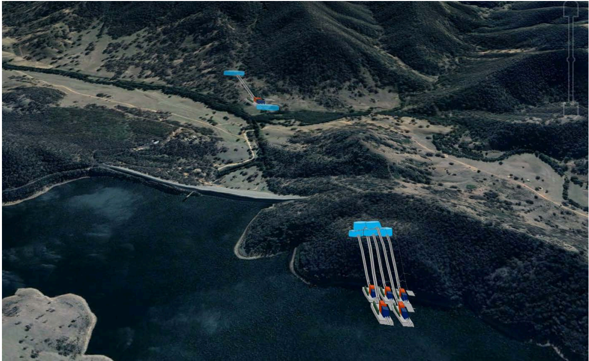
Figure 29: Google earth site location with Floating MPHEs overlay with a scaled (5 x 2MW) 10MW deployment. Upper reservoir 651m and lower reservoir 546m giving 105m elevation difference.
