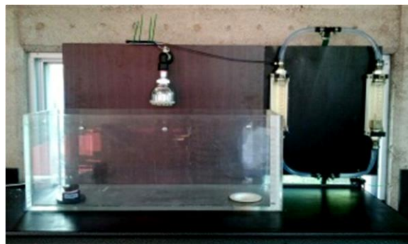
Figure 15: Parallel flow meters and collection tank.
