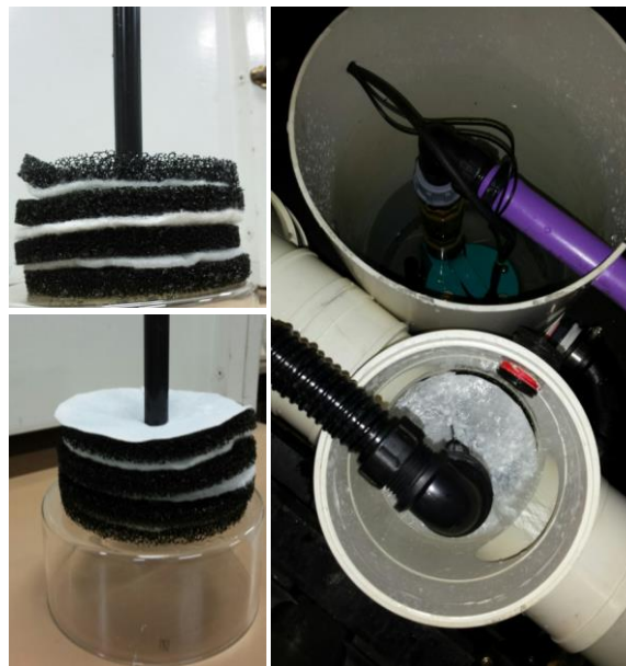
Figure 27: Filter clogging experimental design and setup.
