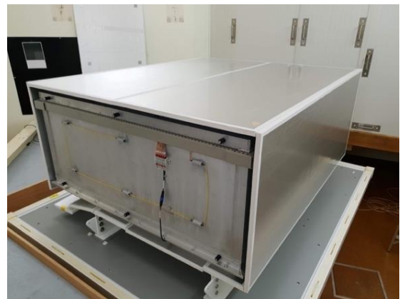
Figure 13: A foam panel has been removed to reveal a heater circuit on one of the internal enclosure panels. The external enclosure walls have been removed.
