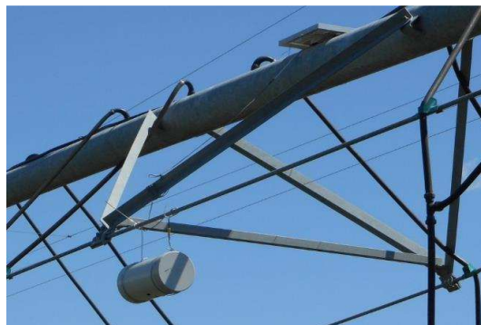
Figure 1: Smartphone on irrigation machine for on-the-go imagery collection
