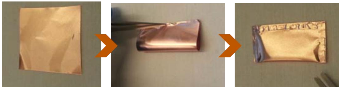
Figure 2.4: Photographs showing a few steps for forming a copper enclosure substrate. Images were taken by Dr. Yufeng Hao (permission granted by Springer Nature). 42
