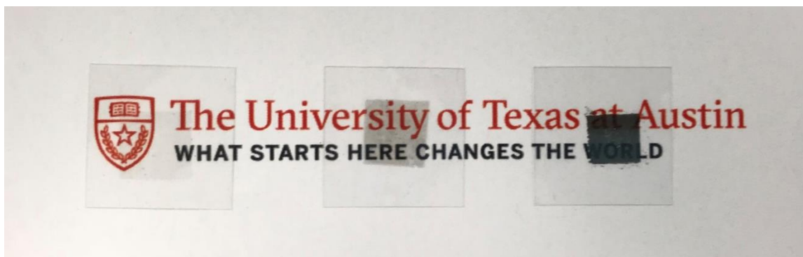
Figure 2.8: Photograph of graphene grown on pure copper (left), 90-10 Cu-Ni alloy (center), and 70-30 Cu-Ni alloy (right). Each layer of graphene absorbs ~2.3% of incident light and the darker films represent thicker multilayer graphene grown on substrates with increasing Ni content, which has high carbon solubility.
