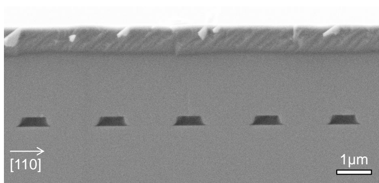
Figure 4.3: Cross-sectional SEM image showing high-quality embedded 300nm tall dielectric gratings in GaAs.
