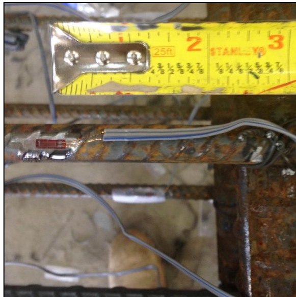
(b) Strain gage application
