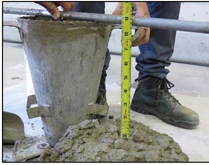
(a) Slump Test
