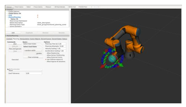
Figure 5.1: Rviz is the 3D Visualization tool used to command the UR3 Robot
