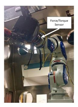
Figure 5.3: Yaskawa SIA5D with F/T Sensor
