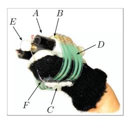
Figure 2.4: Proposed design for a wearable haptic device. The authors specify the items in the diagram as: static platform (B), three motors (A), mobile platform (C), three cables (F), three pulleys (E), and force sensors (D) [29]
