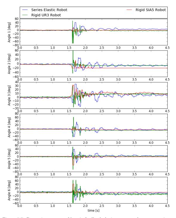
Figure 5.7: Dynamic response of haptic feedback device servo angles to a step input force on the end-effector of each industrial manipulator
