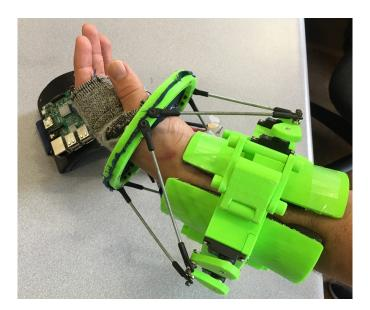
Figure 1.6: Gough-Stewart Platform as a wearable haptic feedback device
