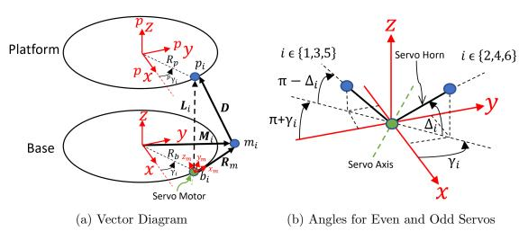
Figure 3.3: General configuration for the  $i^{th}$  servo motor on a rotary actuated GSP
