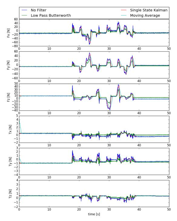
Figure 5.6: Digital Signal Processing of the UR3 wrench signal with random forces and torques applied to the end-effector
