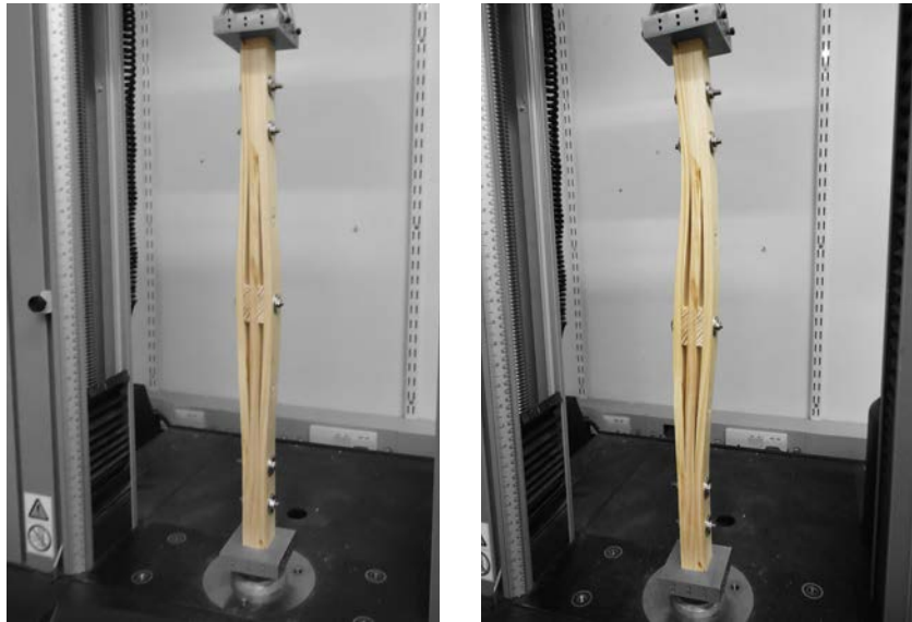
Figure 3.25: Before and after compression testing of a 1:5 model of a split stress-laminated column with a built-up centre.
