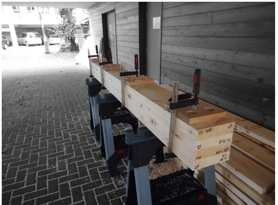
(d) The bearing plates are finally positioned and clamped in the assembly for drilling.
