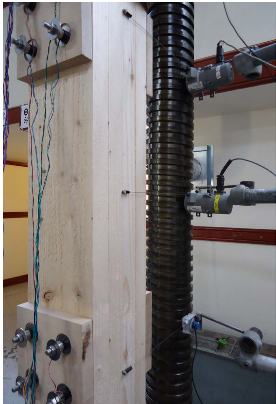
Figure 5.10(a) above left, (b) above right, and (c) right: positioning of the LVDTs for measuring the displacement of the (a) top and (b) bottom plates. (c) Arrangement of wire gauges along the column for measuring lateral deformation and buckling mode shapes.
