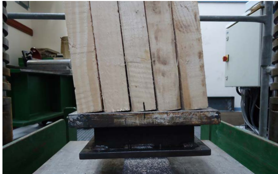
Figure 4.21: Shear deformation between adjacent layers after the onset of buckling.
