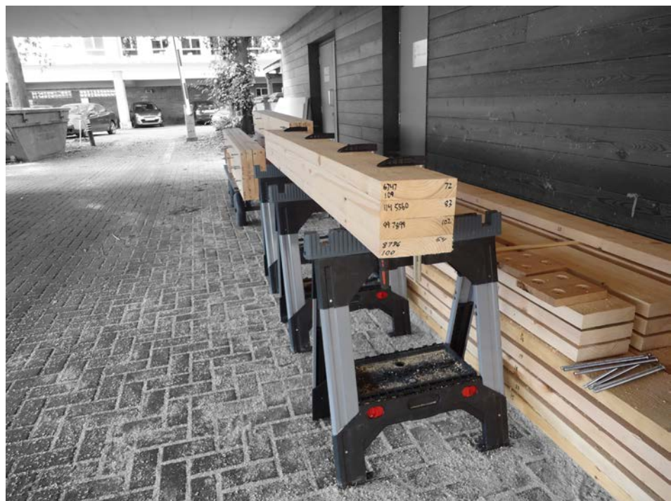
(b) Assembly of individual boards with accurate alignment of the boards' parallel edges.
