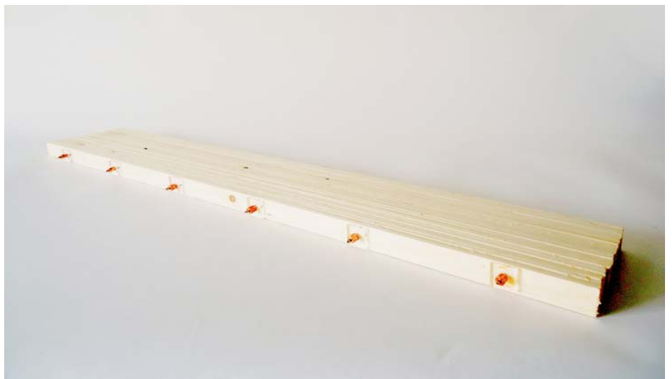
Figure 3.12: Model of a stress-laminated deck or floor panel at a scale of 1:10.
