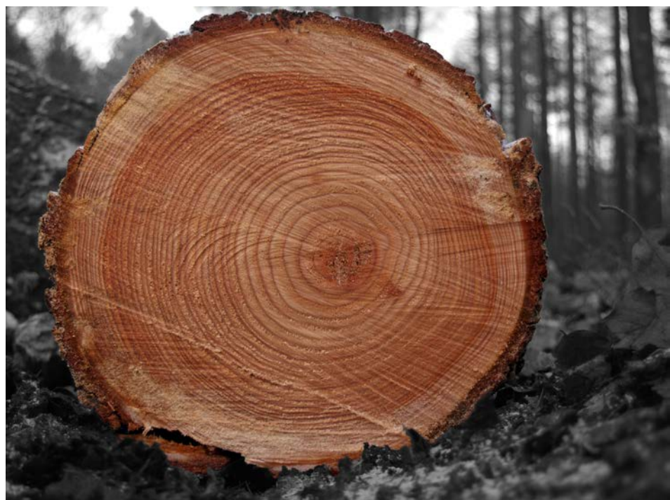
Figure 2.1: Cross-section of a tree illustrating the annual rings and macrostructure of wood. (Photographer: Arnoldius)
