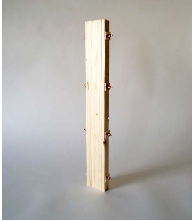
Figure 3.13: Model of a straight stress-laminated column at a scale of 1:10.
