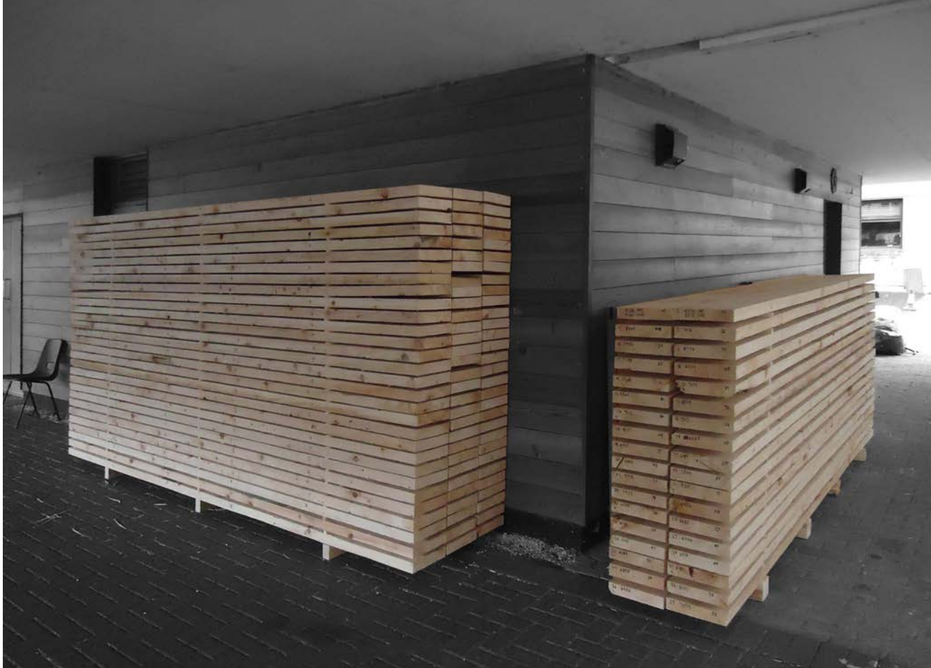
Figure 4.8: Rough sawn UK-grown Sitka spruce supplied by the BSW Timber Limited sawmill at Newbridge on Wye in Wales.
