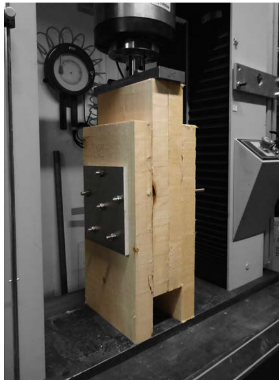
Figure 4.5: Full-scale prototype of a stress-lamination detail in shear testing.
