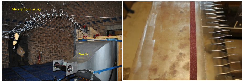
(a) The experimental rig was placed in the aeroacoustic wind tunnel. The flat plate was placed near the exit of the wind tunnel and a microphone array was suspended above the aerofoil to measure the far-field noise. (b) The serrated leading edge was formed by joining the serration insert and the flat plate together. The serration insert was cut according to equation (37) and the parameter b was varied between 0 , \pi , 1.2\pi and 1.5\pi .
