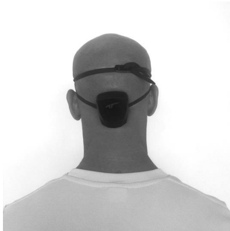
Figure 1. Placement of TritonWear® device fitted directly inferior to the inion, on the occipital bone.
