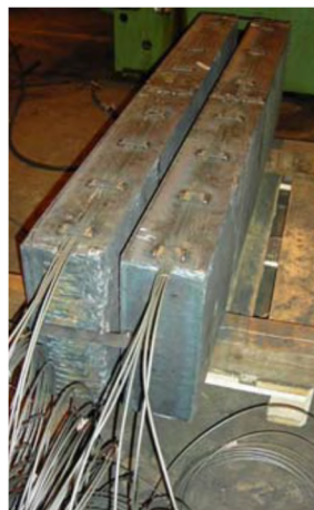
Figure 3. Images of the pilot-scale walking beam furnace (top) and the instrumented slabs with thermocouples (bottom)
