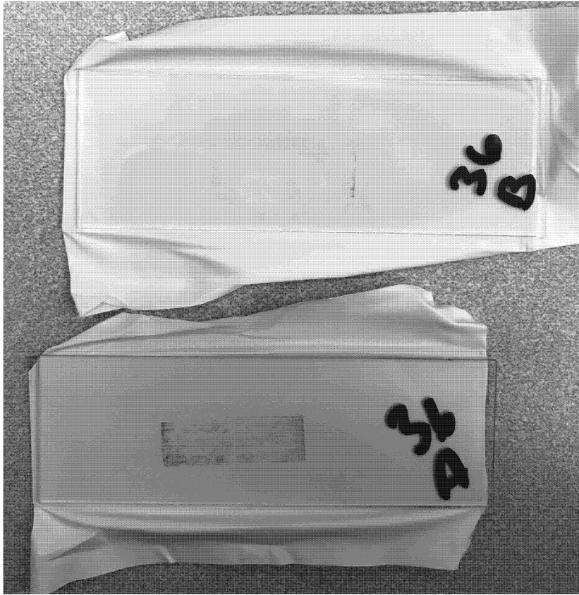
Figure 5.6: Before and After Tape Lifts of Sample 36
