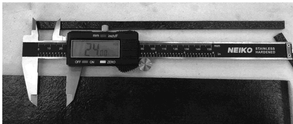
Figure 4.7: Measurement of Sample Length on Water Jet Cut Strip
