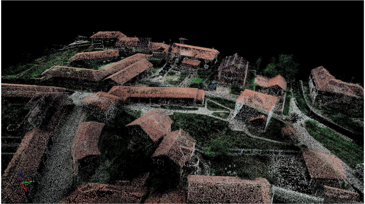
Figure 6. The point cloud through a creation of tie points (Pix4D, 2018).
