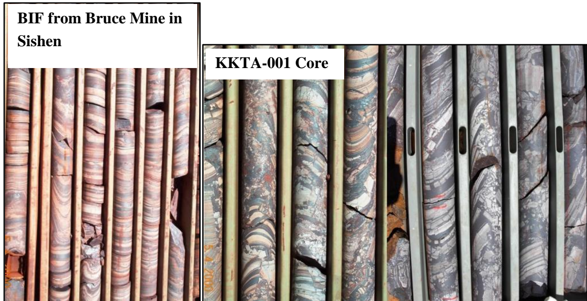
Plate 6.1: Comparison of the Kuruman iron formation from Assmang in Sishen and KKTA001 cores, both these iron formations are micro banded and brecciated.
