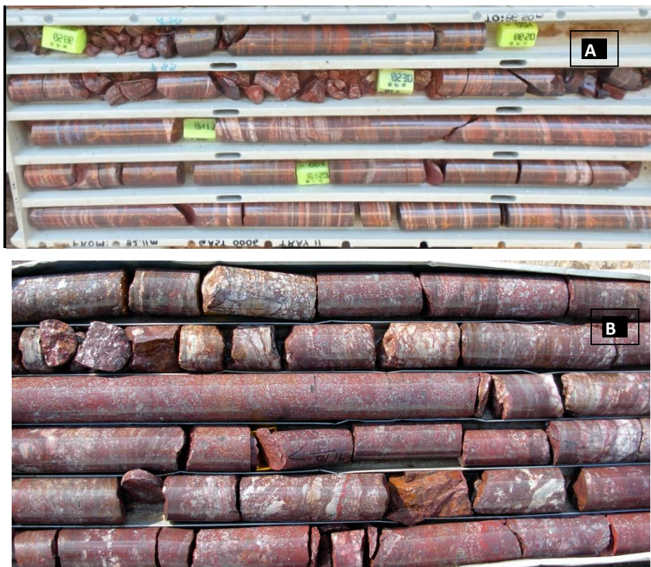
Plate 3.7: (A) Tshitsane Hill BIF, characterised by micro-banded, siliceous and jasperlittic (B) Kgwakgwe chert breccia intersected during drilling characterised by ferruginous matrix, this breccia was underlain by a dolomite unit intersected in the same bore hole drilled to the NE of Tshitsane.
