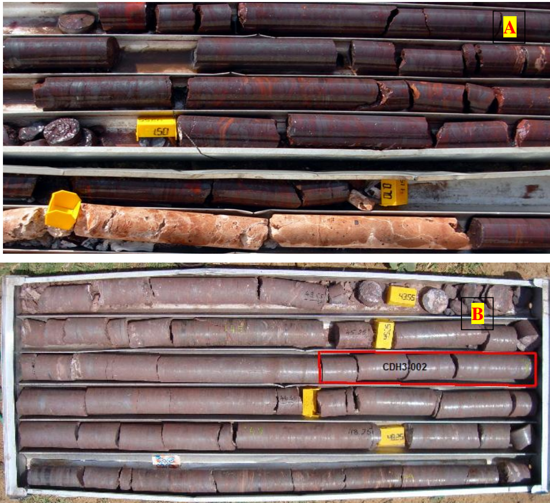
Plate 3.1: A: a mineralised section of the core drilled in the Tshitsane Hill. B: a sampled section of the core.
