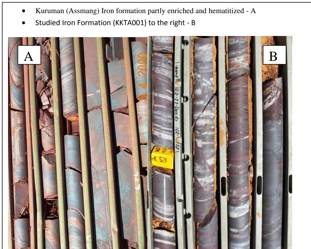
Plate 6.1: Comparison of the Kuruman iron formation from Assmang in Sishen and KKTA001 cores, both these iron formations are micro banded and brecciated.
