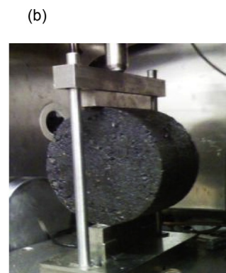
Fig. 6 – Moisture induced stress tester. (a) Conditioning process using MIST in progress. (b) ITS test setup.
