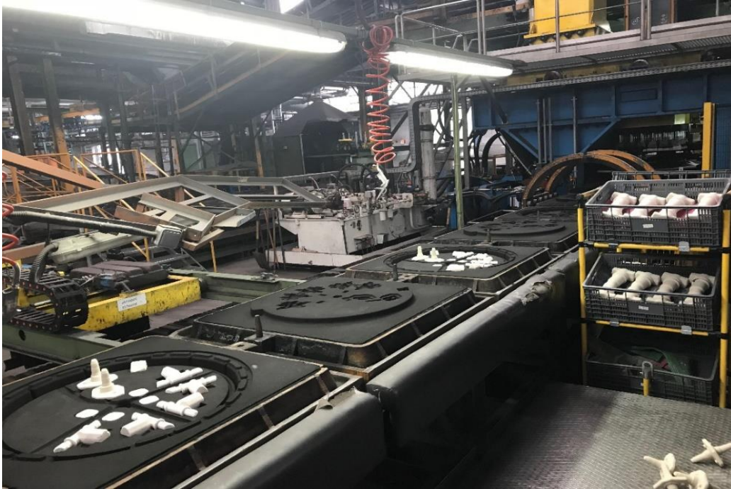
Figure 3.2 – Placed sand cores before iron pouring
