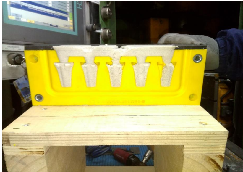
Figure 3.23 – Faulty filling of the core box
