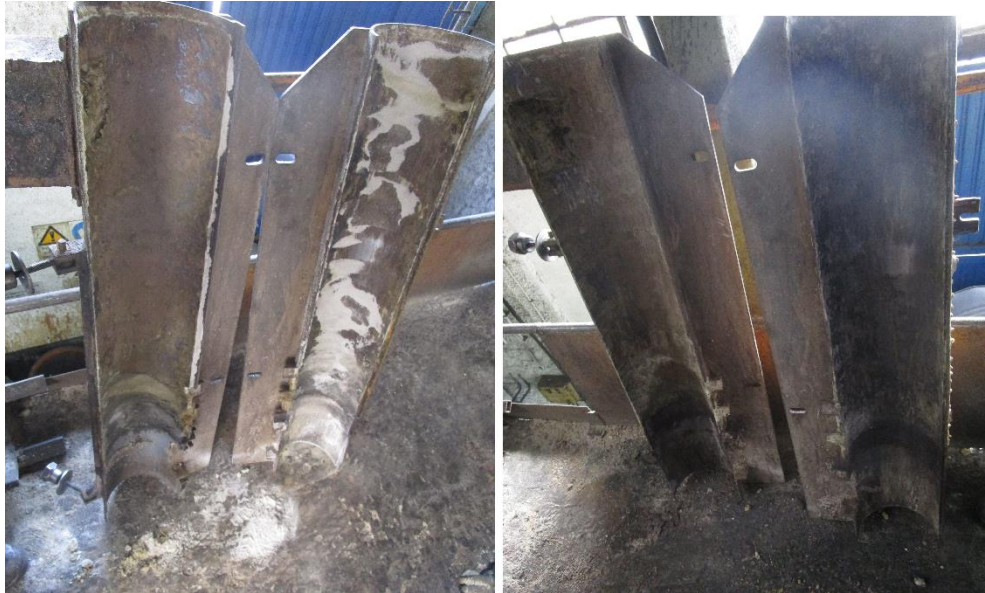
Figure 3.17 – Covers of the mixer before and after intervention
