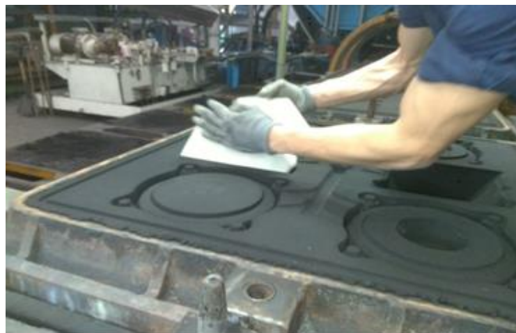
Figure 3.1 – Placement of a sand core in the foundry department
