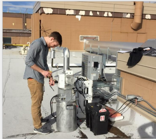
ASR was set up on test roof to get real-time atmospheric measurements
